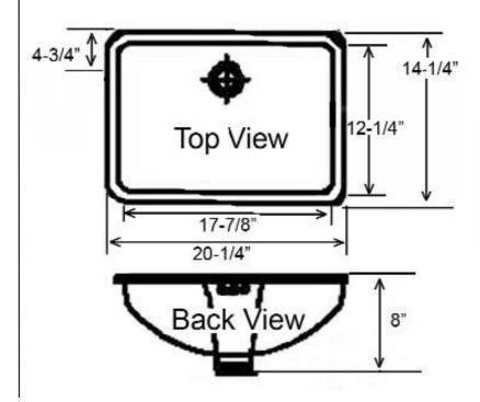
Dimensions of fixture are nominal and may vary within the range of tolerances established by ANSI Standard A112.19.2.2018 Dimensions and specifications subject to change without notice.
